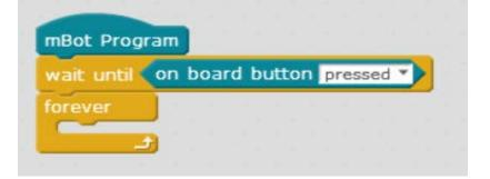
Don't run it yet, but let's just look at it for a second. What does it do? Well, basically what it does is when the code is uploaded to the mBot it will start running. This is awkward if the robot just runs off when you aren't ready, so we wait for the button to start.
